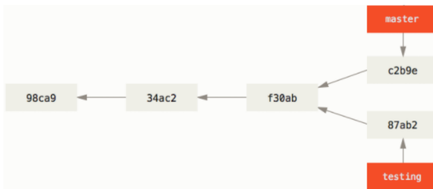
Figure 2.4: After both branches have committed a different commit. Two commit objects reference the same parent commit.
