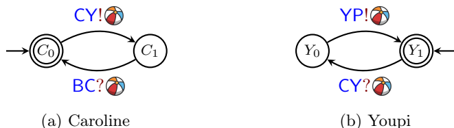
Figure 1.4: State machines modelling the local perspectives of two players for the state machine in Figure 1.2 .
